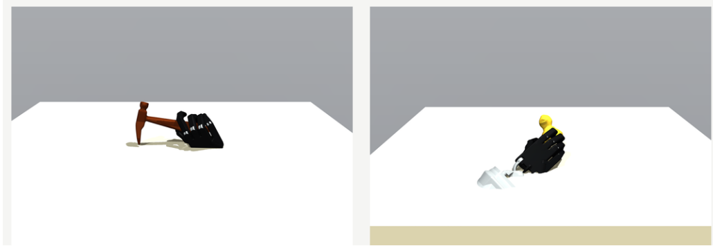
Figure 22. BODex-Shadow failure cases. Panels 2 and 3 illustrate a common failure mode of random/geometric initialization: without a human prior, the optimizer can place the Shadow wrist into the table while pursuing local hand-object contact, producing wrist-table collision before a usable grasp configuration forms.
