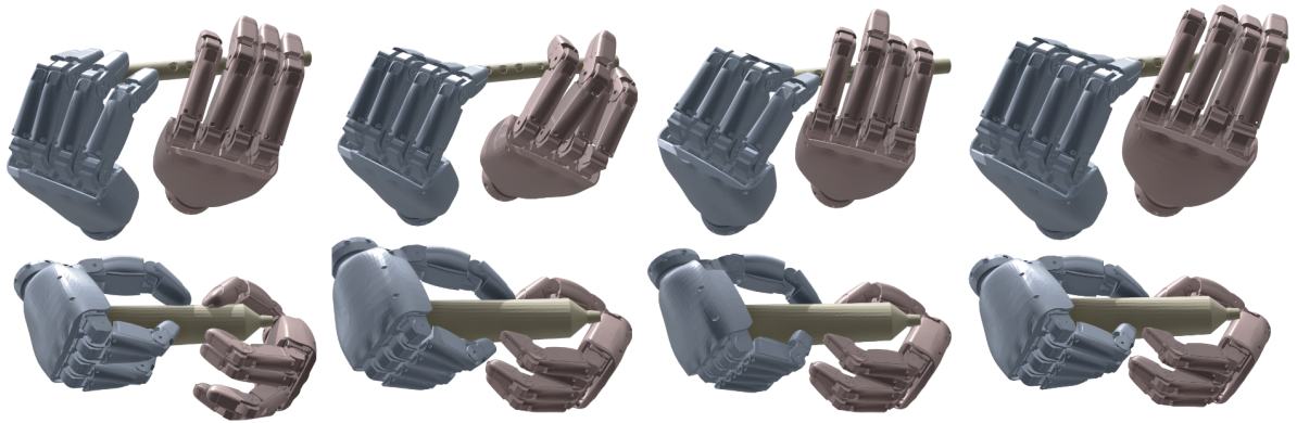
Figure 10. Selected in-grasp manipulation trials from validated keyframes. These simulated sequences test asynchronous coordination, where one hand maintains support while the other applies directional manipulation forces.
